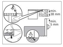
If you use a protection box (the additional accessory<sup>1)</sup>), the front airflow space of 5 mm and protective floor directly below the appliance are not necessary.
